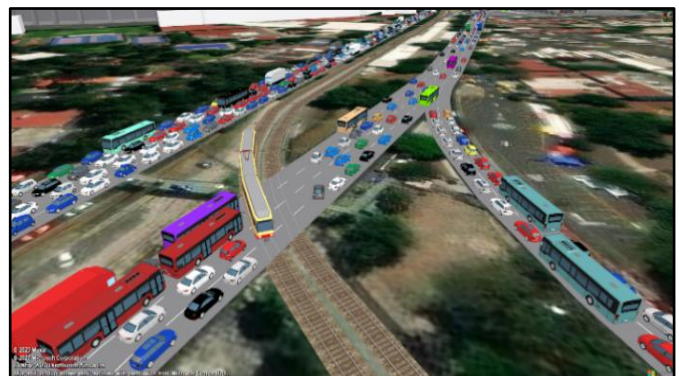
Figure 13. Simulation of dynamic of vehicles at the Azteca stadium, using Vissim™ software.
