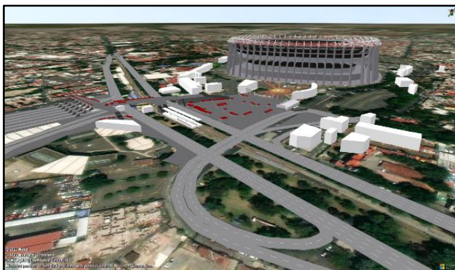
Figure 10. Simulation model of main streets around Azteca stadium, using Vissim™ software.
