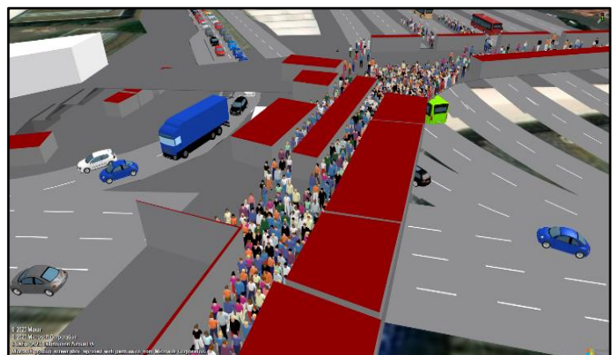
Figure 12. Simulation of dynamic of pedestrians at the Azteca stadium, using Vissim™ software.
