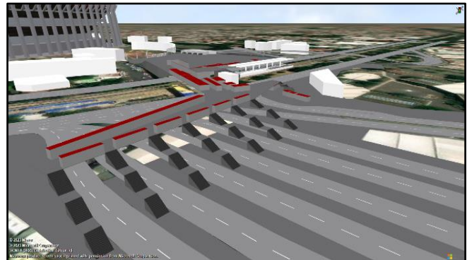
Figure 11. Simulation model of main bus stations around Azteca stadium, using Vissim™ software.
