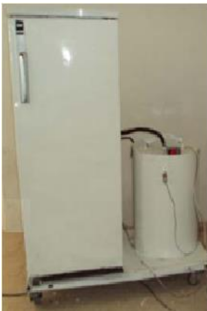
Figure 1. Household refrigerator for water heating
