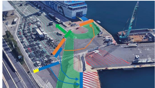
Figure 4. The organization of entry and exit flows and waiting queues for boarding
