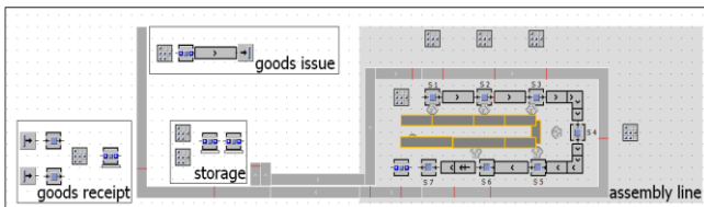
Figure 2. Representation of the used U-cell assembly line simulation model
