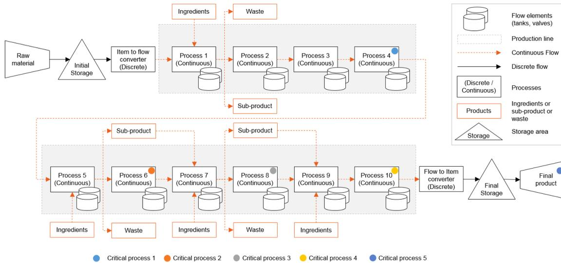
Figure A.1. Conceptual diagram of the discrete and continuous processes developed in Simio®
