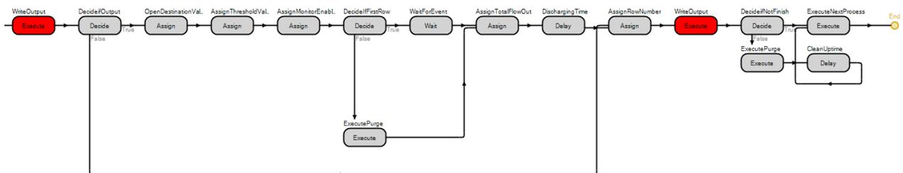
Figure A.3. Internal logic for processing and discharging operations developed in Simio®
